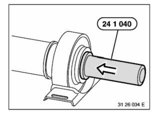
Drive on centre mount with ball bearing using Special Tool 24 1 040.
